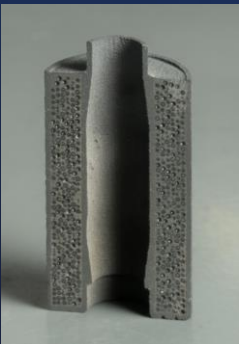
TRISO Encased in Ceramic Matrix
