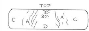
Upset disk, such as might be used for fabrication of a head
