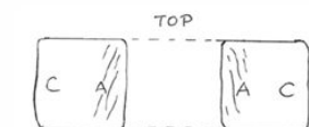
Forged ring; the center is removed (trepanned), significantly reducing the volume of macrosegregation
